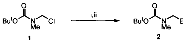
Scheme 2. Reagents and conditions: i, Li, DTBB cat. (2.5 mol %), \text{E}^+ = \text{Me}_3\text{SiCl} , \text{Bu}^i\text{CHO} , \text{Bu}^t\text{CHO} , \text{PhCHO} , (\text{CH}_2)_4\text{CO} , \text{Et}_2\text{CO} , \text{PhCOMe} , \text{Ph}_2\text{CO} , THF, -78^\circ\text{C} , 2 h; ii, \text{H}_2\text{O} .
